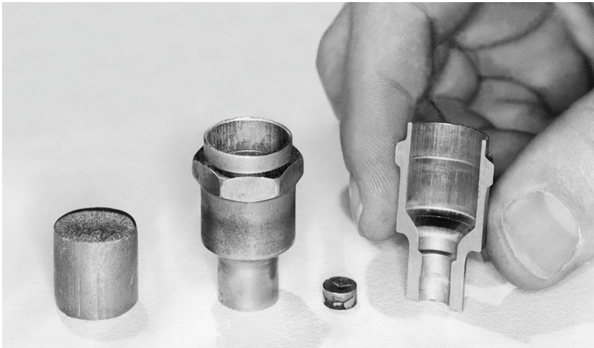
Figure 15.12 Production steps for a cold extruded spark plug. Source: National Machinery Company.
